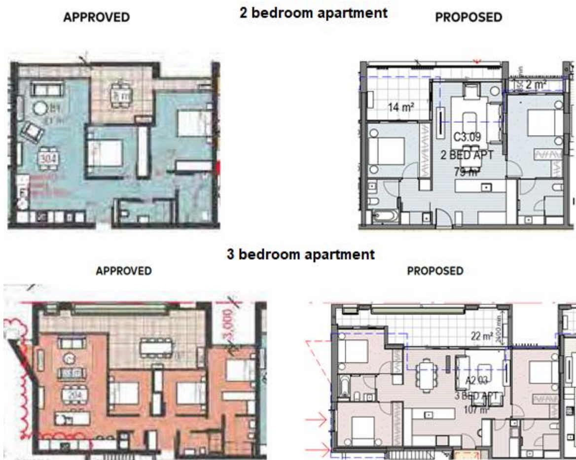
Figure 2: Changes to apartment layout – living area off balcony, entry to living zone, and separate bedroom areas. The blue dotted line outlines the changes in the apartment layout resulting in increase in floor area. The increase is within the building envelope and complies with the ADG requirements in terms of layout and balcony size.
